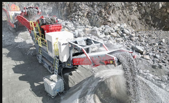
A new electric cone crusher, QH443E, takes a significant step towards bridging the gap between tracked mobile, wheeled portable, and stationary plants, by combining electric drives and track mobility on a single platform.
